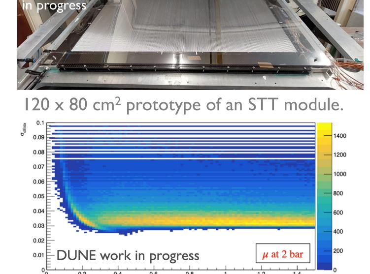
Measured prototype dE/dx resolution
