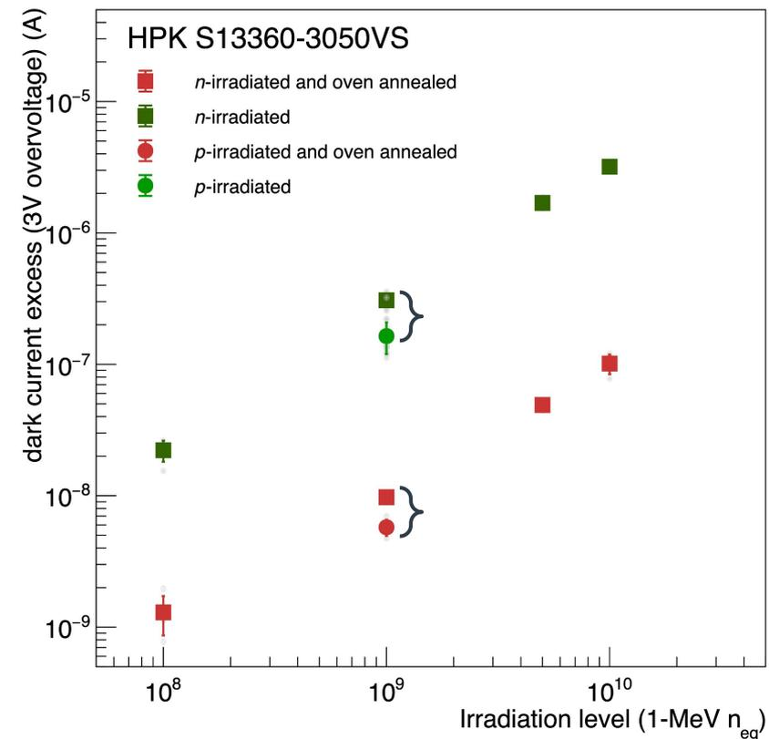
A bit of care needs to be put in interpreting the results of the neutrons as a factor 2 in damage has been found between, using NIEL scaling normalisation
