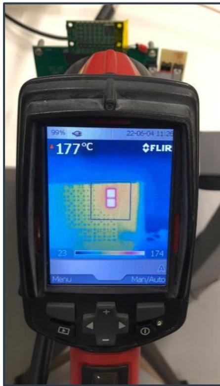
Online annealing done with sensor in forward bias, delivering  $\sim 1$  W/sensor
