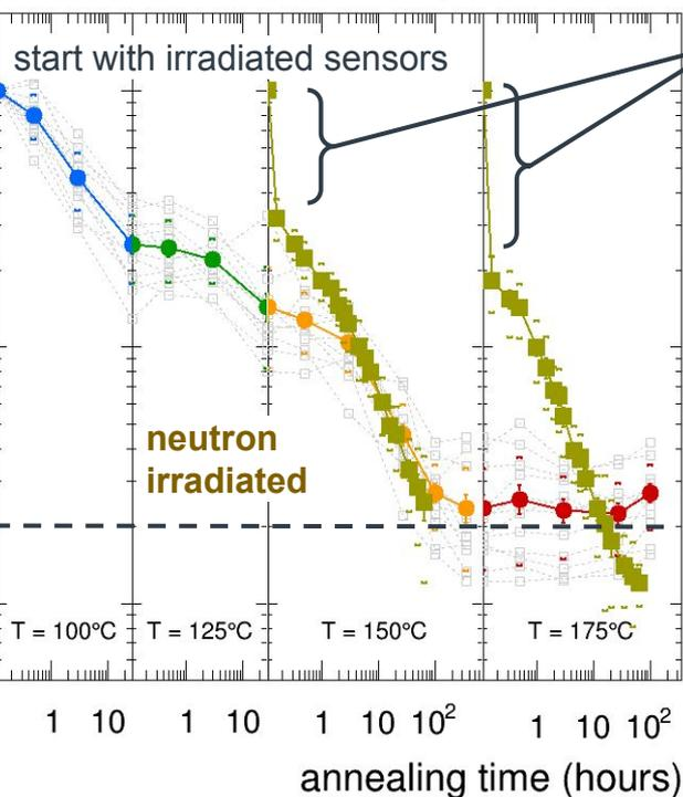
Both annealing samples show a substantial recovery (70/80%) in a small time (10 min)
