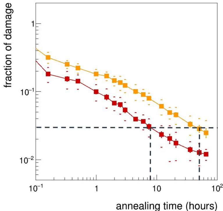
Both annealing samples show a substantial recovery (70/80%) in a small time (10 min)
