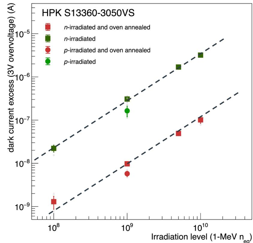
A bit a care needs to be put in interpreting the results of the neutrons as a factor 2 in damage has been found between, using NIEL scaling normalisation
