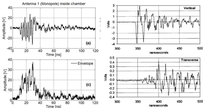
Examples of time-domain signals measured with Antennas inside the vacuum chamber of the ABC and Vulcan facilities
