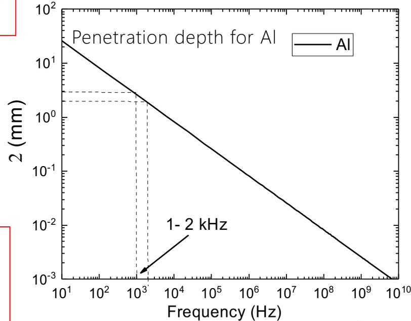
The 2-3 mm Al thickness can attenuate EMP with frequencies down to 1-2 KHz
