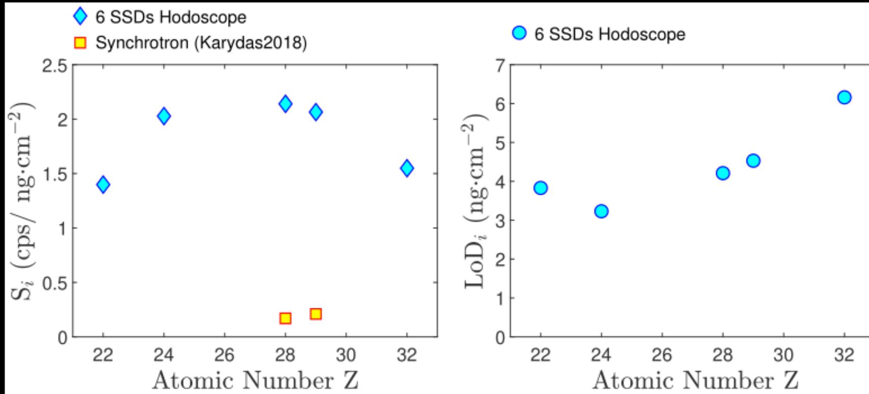
Figure of merit of the upgraded system in comparison with a typical single-detector set-up available in a synchrotron facility
