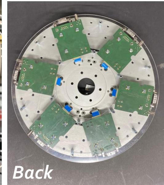
The 3D detector array allows us to **increase the throughput of the fluorescence radiation** ensuring enough statistics for pixel XRF spectra at short dwell-time
