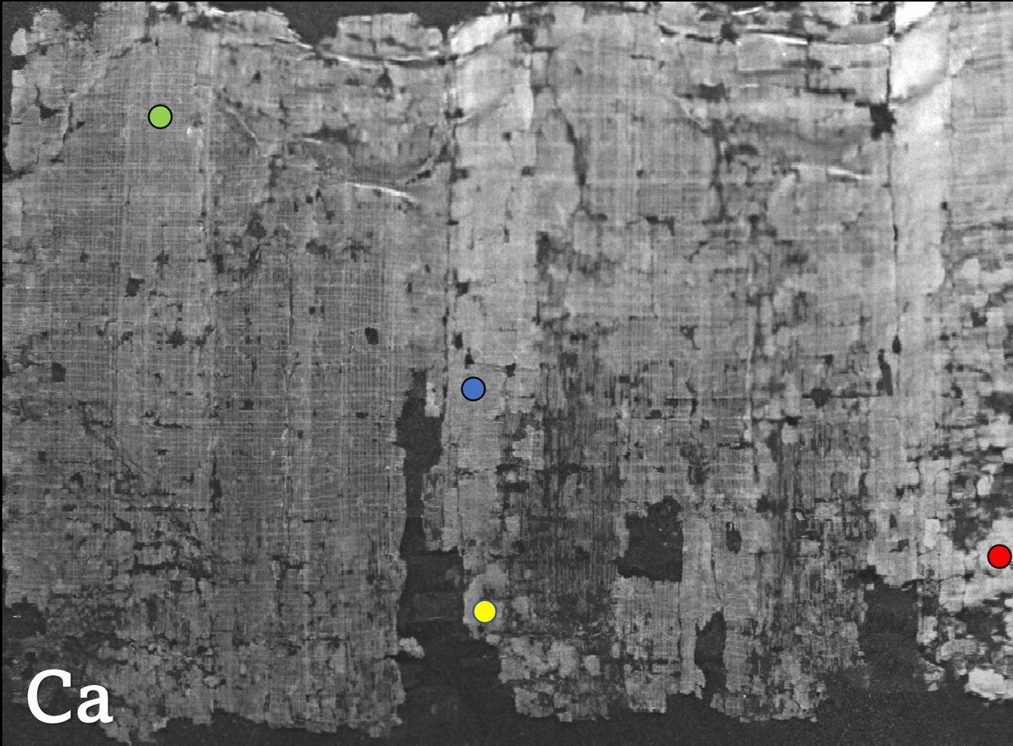
Ca-K $\alpha$  fluorescence signal along the stratigraphy for the identification of overlaid/underlaid layers
