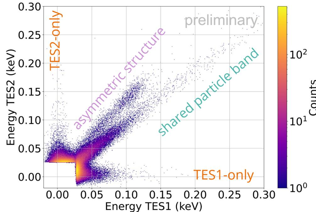
Additional structure with an asymmetric energy sharing between two TES.
