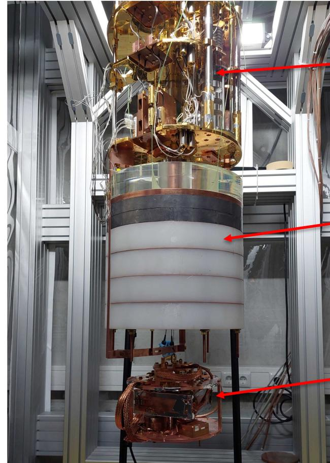
Cryostat (10mK) and readout
