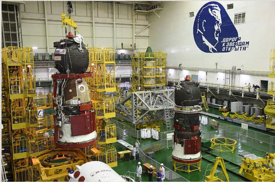
Building 254, assembly of Soyuz/Progress
