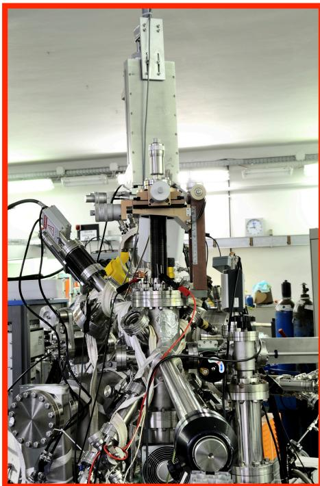
The 2010 has been also devoted to the optimization of a 'state of the art' **spectroscopic chamber**, in order to be able to do **angle resolved photoemission experiments, also at low temperature**. This system has been **tested** at length during this year and **a fast load-lock system has been implemented** in order to be able to change samples to be studied with SR without breaking vacuum.
