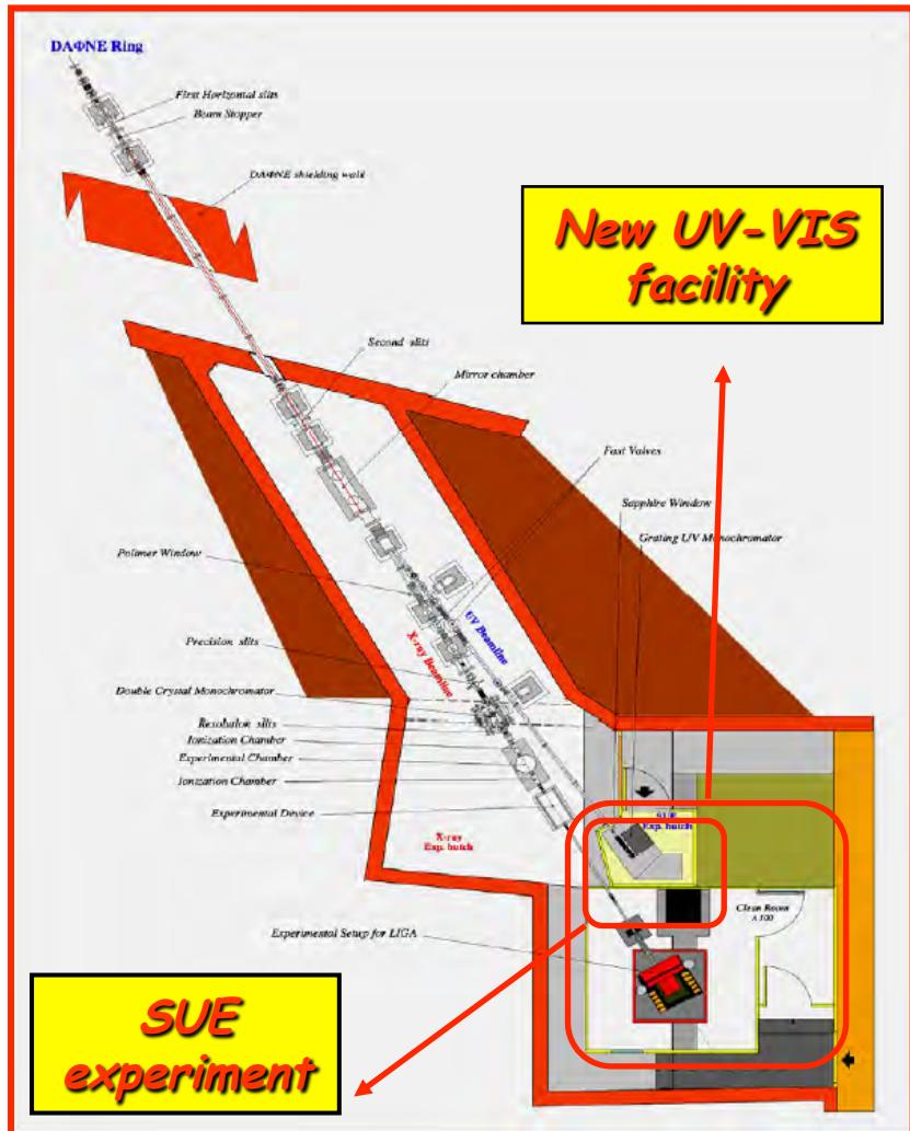
Wiggler UV branch line-deflection by a grazing incidence gold coated mirror
