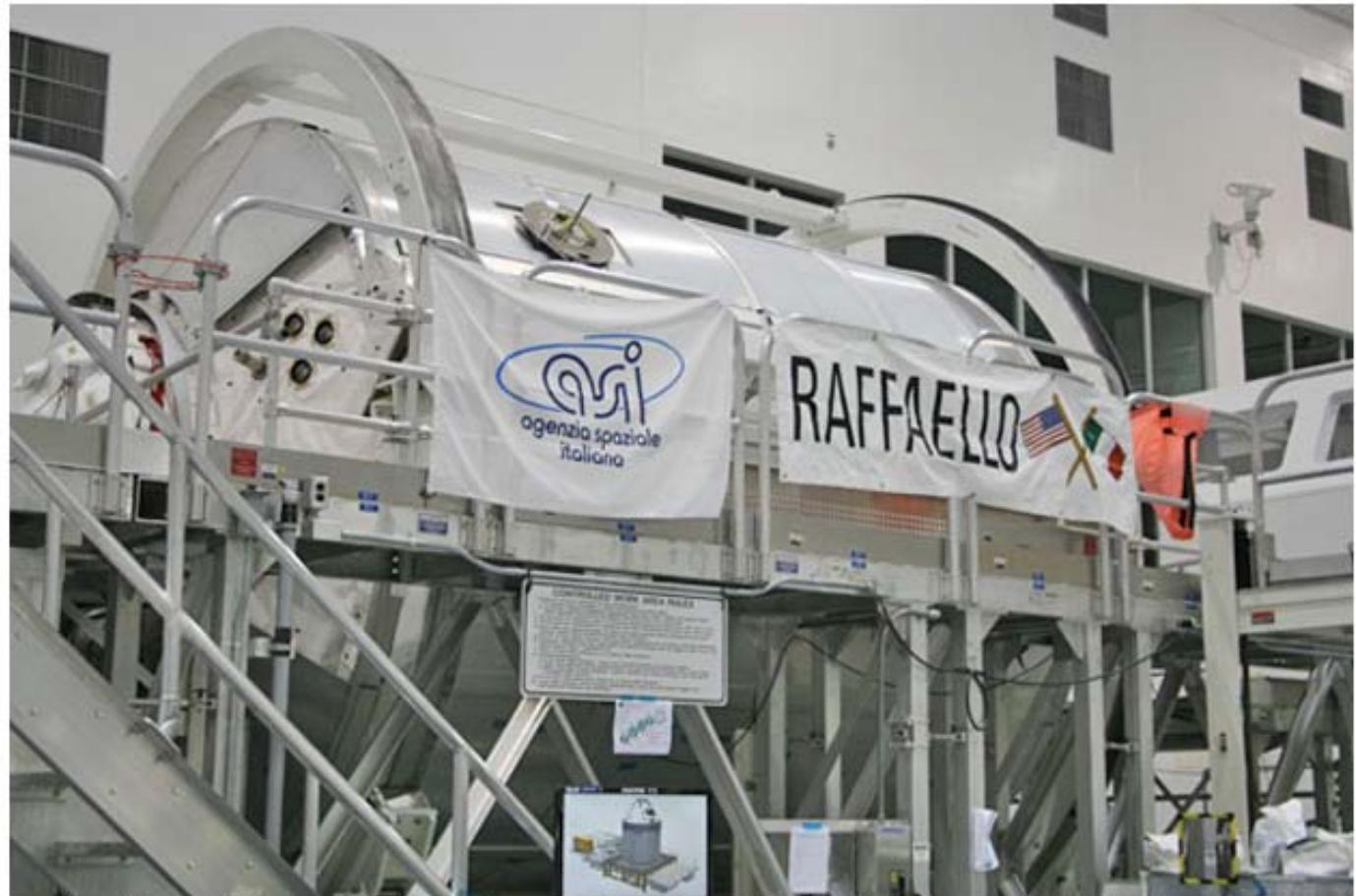
Raffaello multipurpose logistics module (MPLM) inside the Space Station Processing Facility (SSPF). On the very last flight of the Space Shuttle program, Raffaello will be delivered to the ISS by Space Shuttle Atlantis on the STS-135 mission. Robotic arm grapple fixture at top, left. The cylindrical module is approximately 21 feet long and 15 feet in diameter, weighing almost 4.5 tons. It can carry up roughly 25,000 pounds of cargo to orbit.
