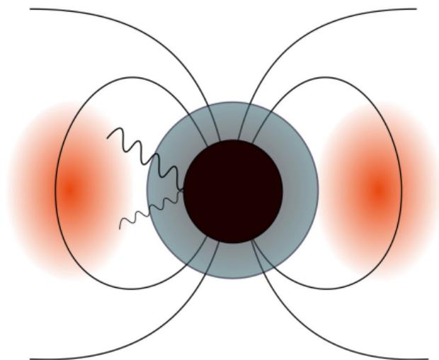
Schematic illustration of the instability. The axion boundstate (orange) mixes with a photon mode which is then amplified by scattering off the rotating magnetosphere (grey). The photon energy is then deposited back into the axion sector.
