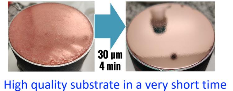
In collaboration with CERN, it will be investigated if PEP provides a reduction in surface resistance of SRF coatings and scalability to 1.3 GHz elliptical cavities.
