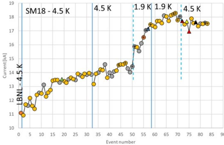
It trained A LOT. It reached 100% of maximum field at 4.5 K. No conductor degradation occurred from handling, assembly, powering, or thermal cycling.
