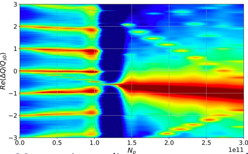
Due to the updated parameter list, the bunch population is higher and, even if the TMCI thresholds are similar, with the 30 mm radius the instability is much stronger.
