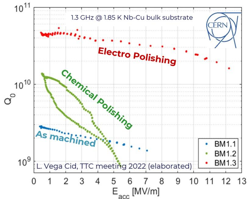
Roughness and defects reduction by **surface treatments are mandatory** for a good and uniform SRF coating
