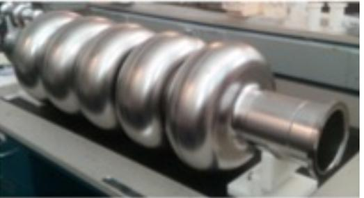
800 MHz segmented design, based on PIP-II
