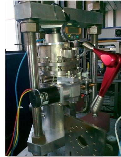
**LASA tuner test setups, room T and cryogenic**
