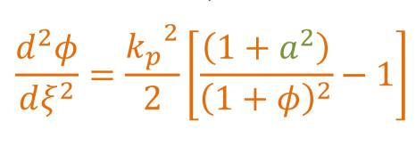
The laser field is represented by the normalized vector potential  $a = \frac{|e|A_{\perp}}{m_0 c^2}$
