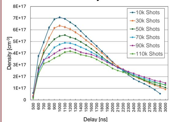
Fig. 7: mean density over delay for different lifetimes
