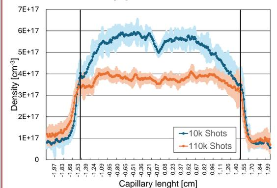
Fig. 6: Profile density for 1mm diameter
