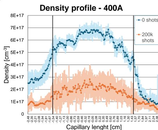
Fig. 2: Profile density for 2mm diameter
