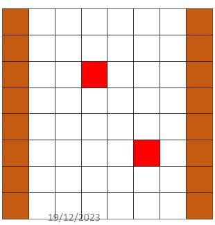
CASE 1: LOW threshold verified on two or more pixels. Hitmap generation. CASE 3: Light pollution. Hitmap generation. No data digitization.
