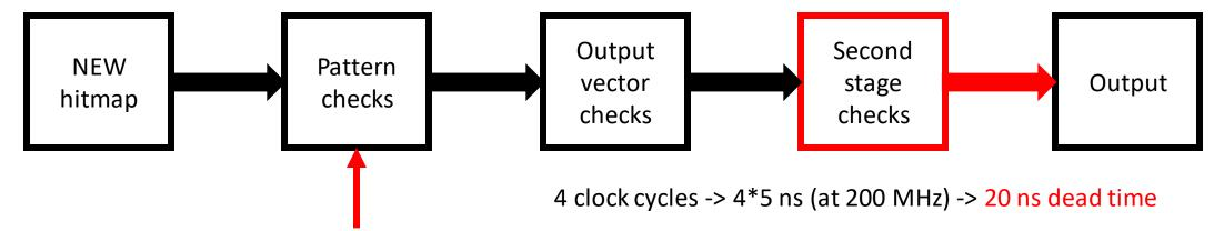
Modification required to account for the additional ASICs -> higher FPGA utilization
