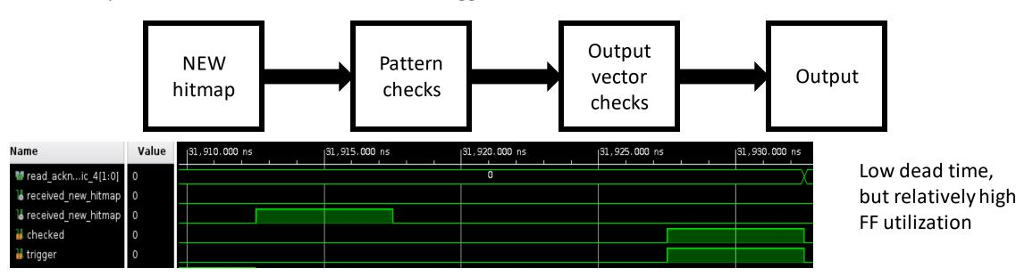
3 clock cycles -> 3\*5 ns (at 200 MHz) -> 15 ns dead time In the FPGA, much less than the transmission time of a hitmap packet
