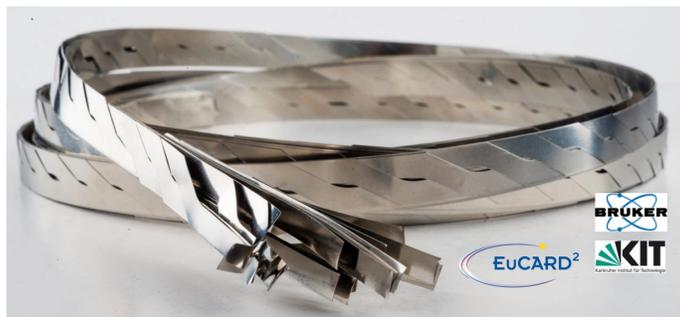
YBCO High-Temperature superconducting magnets
