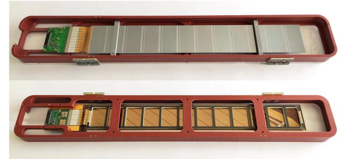
AMS-02 ladder made of 12 double-sided  $40 \times 70$  mm<sup>2</sup> silicon microstrip sensors
