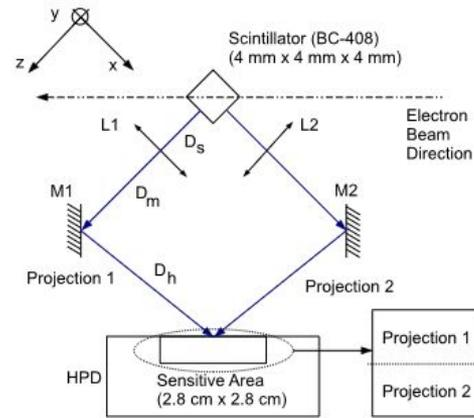
**Fig. 4** Schematic view of the setup used for the measurements. It consists of a plastic scintillator, two lenses (L1, L2), two mirrors (M1, M2) and the HPD. One projection of the electron track in the scintillator is imaged on the top half of the HPD and the other on the bottom half.  $D_s = 34\text{ mm}$ ,  $D_m = 25\text{ mm}$ ,  $D_h = 77\text{ mm}$
