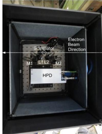
**Fig. 5** A photograph of the setup used for the measurements. The detector and the optics were shielded by two layers (black plastic, dark paper board) from external optical photons. The beam direction is shown in the photograph
