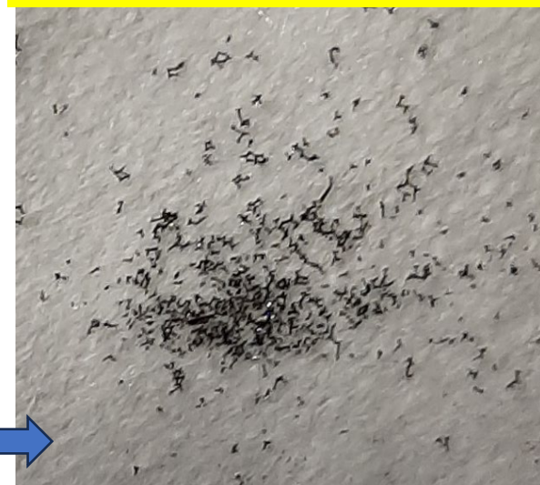
Carbon ERG fibers: after vacuum treatment
