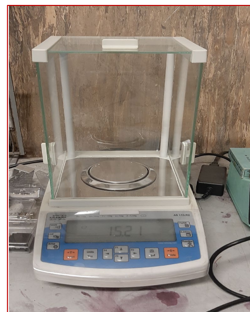
Analytical balance (Radwag AS 110-R2): Res 0.1 mg
