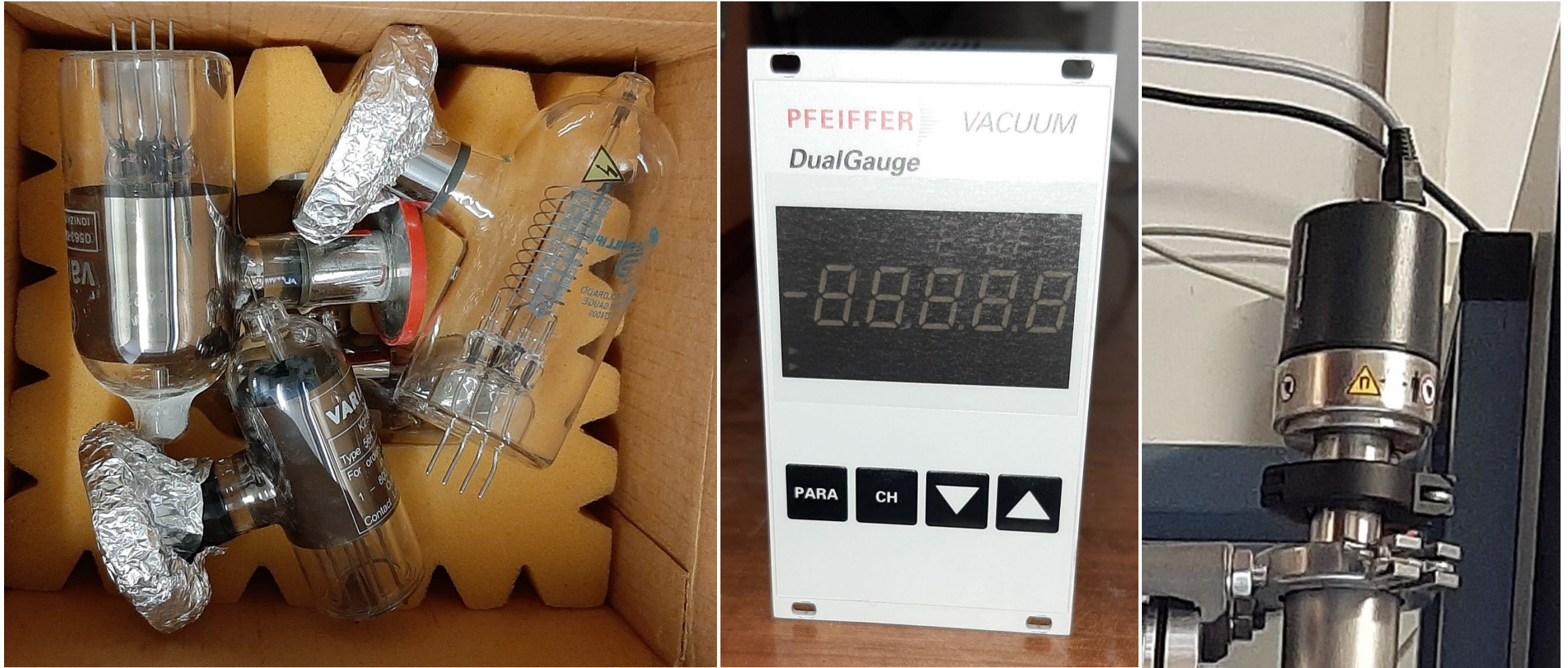
Fig: Vacuum gauges and display unit
