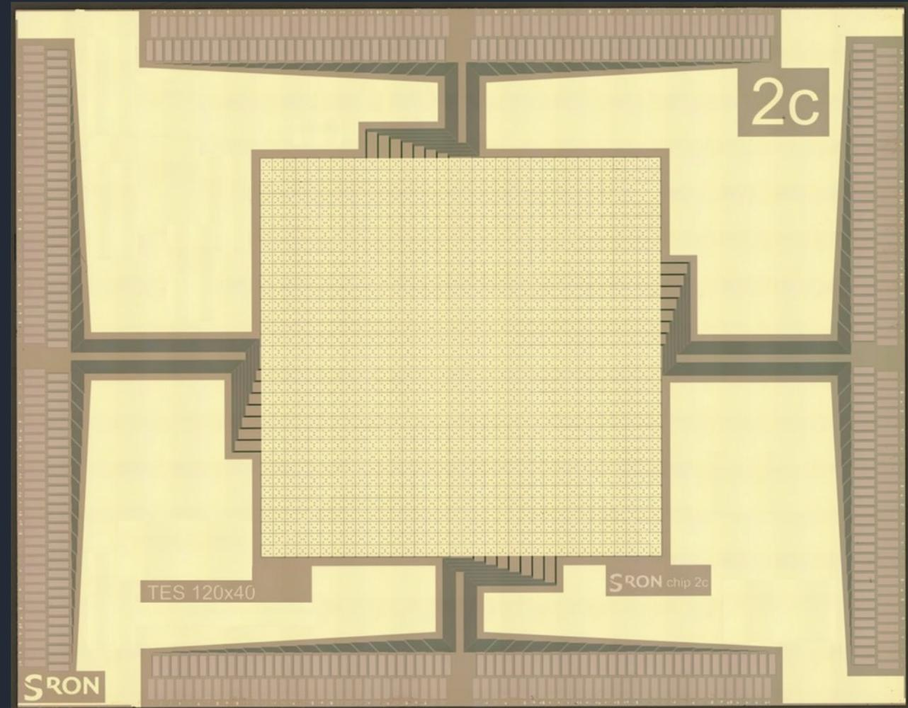
Final chip SRON 32x32 X-ray microcalorimeters
