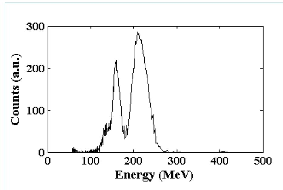
First results focusing less than 1/10 of the maximum LASER power in a supersonic gas-jet at about 10Atm of N<sub>2</sub>
