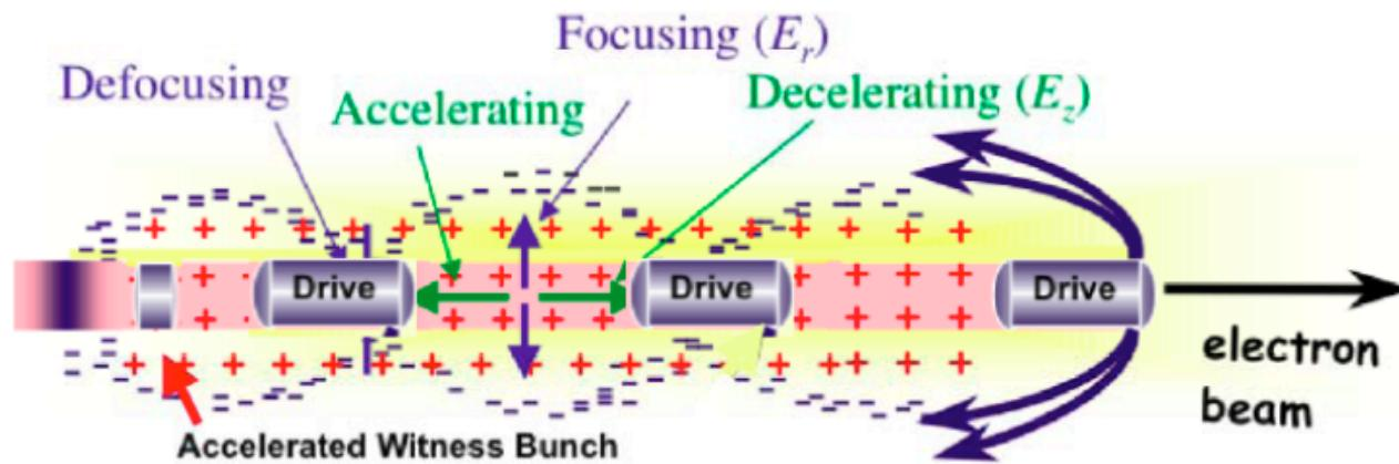
Due to the high control on the LINAC photoinjector we intend to accelerate electrons in a plasma wave resonantly excited by a train of e-bunches
