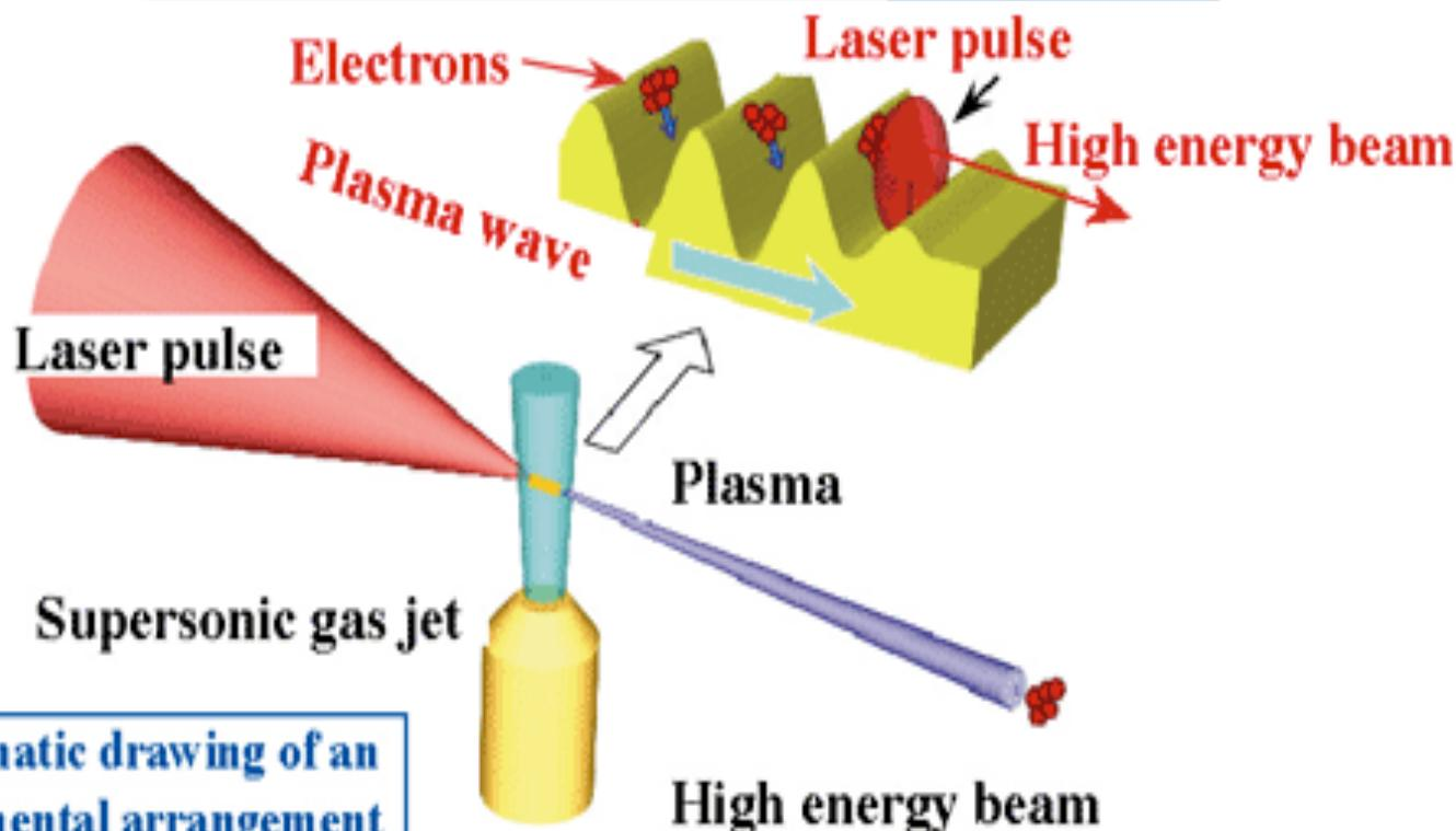
A schematic drawing of an experimental arrangement
