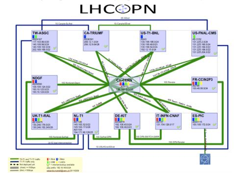
A fully redundant **LHCOPN** for T0-T1 (and T1-T1) And soon: "**LHCONE**" for T2/3
