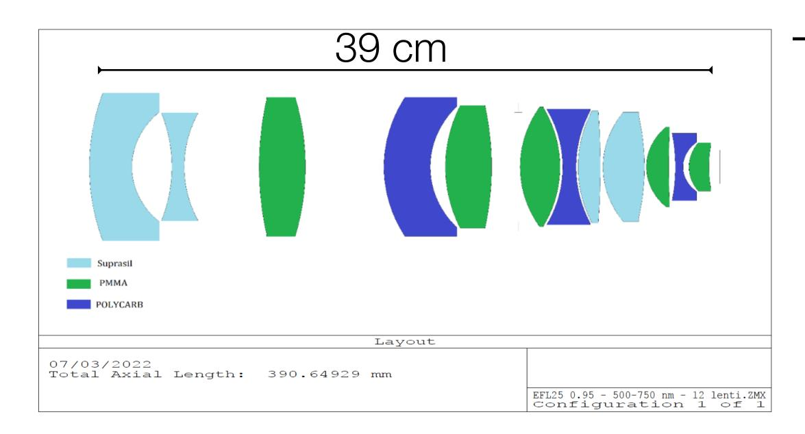
Use of 3 different low radioactive materials should will provide the requested optical performance
