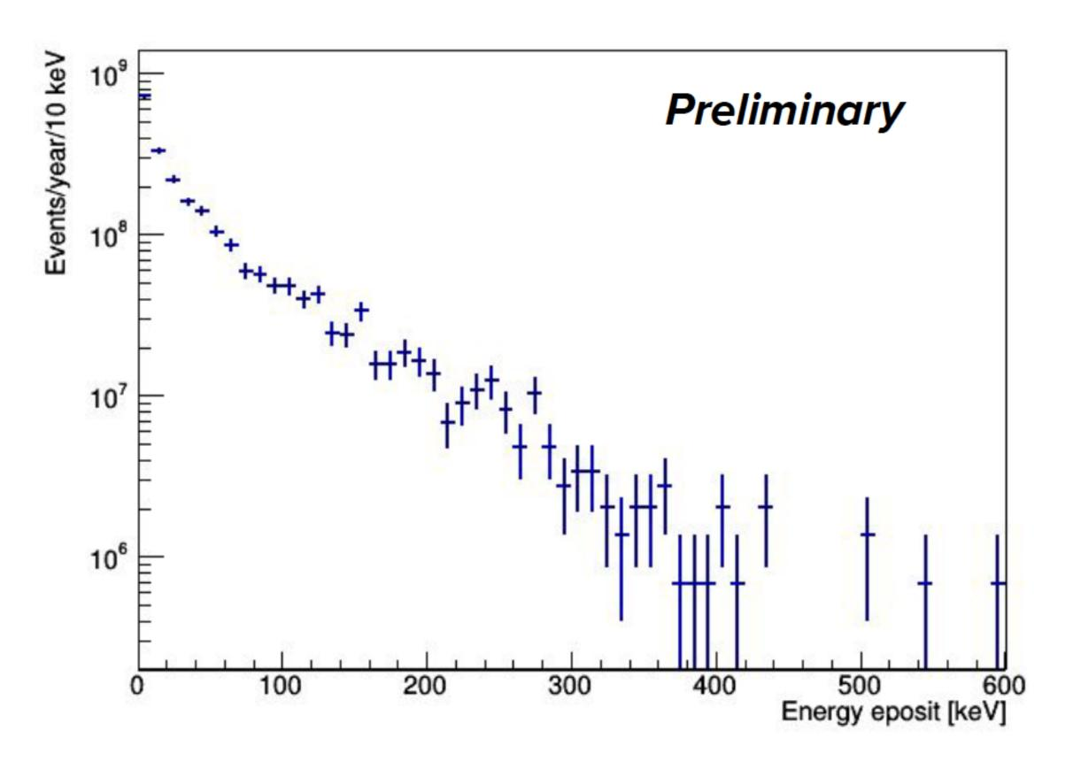
Average gamma flux attenuation of 1 m water + 10 cm Cu  $\rightarrow$  ~5 x 10<sup>-6</sup>
