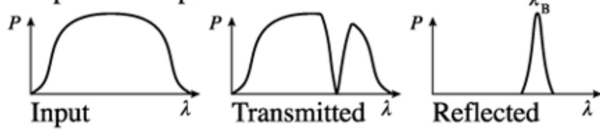
Fiber Bragg Grating (FBG) sensors have been so far mainly used in high energy physics as high precision positioning and re-positioning sensor and as low cost, easy to mount and low space consuming temperature sensors. FBGs are also commonly used for very precise strain measurements
