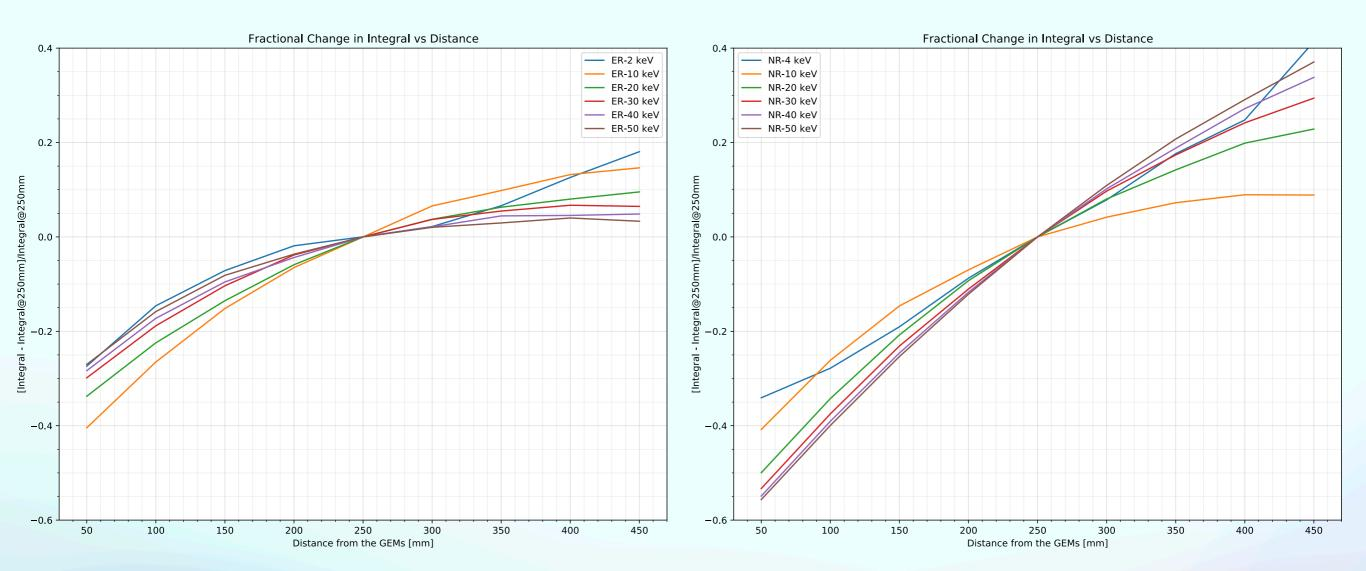
Change in light integral for ER at all the energies with respect to the light integral at 25 cm away from the GEM is between ~[-30, 10]%.
