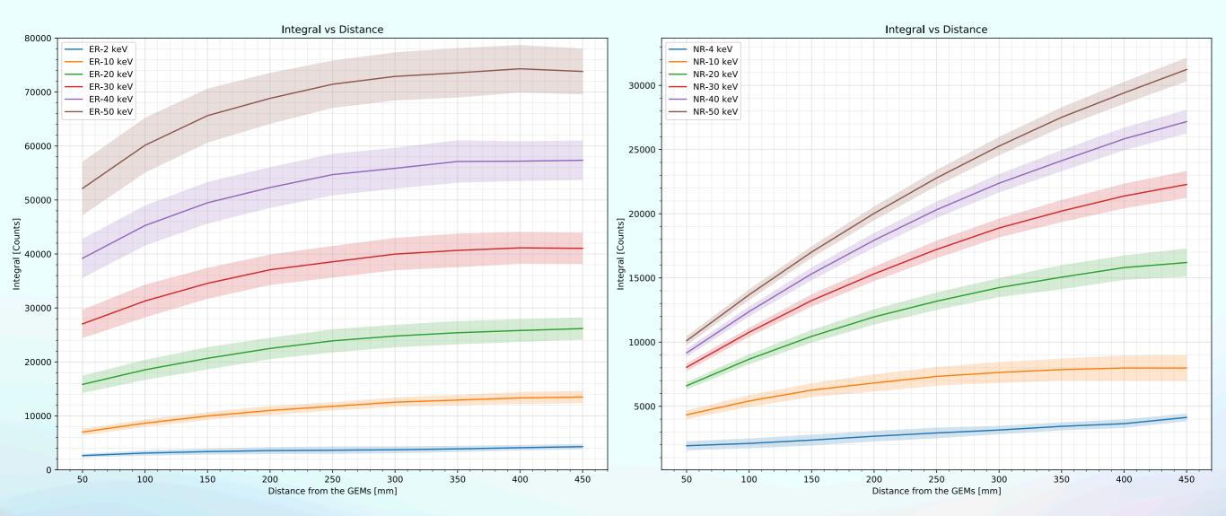
Light integral ER data reaches a plateau after 25 cm while as light integral NR data increases as we go away from the GEMs at all the energies.
