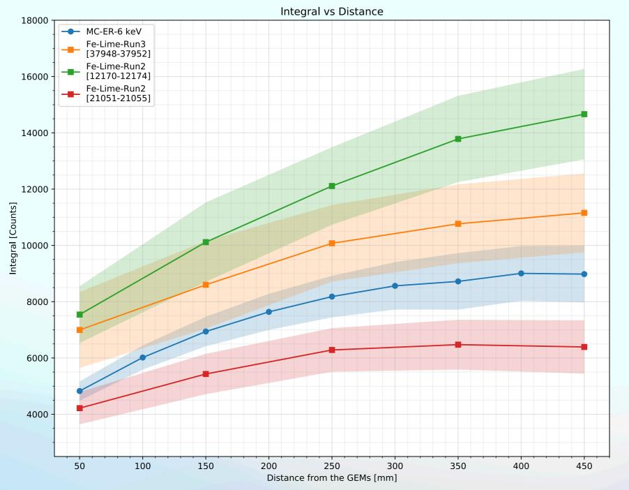
• Light Integral comparison of MC at 6 keV and Fe calibration data different runs. All the data sets have different light yield, so need to be corrected to match the MC.
