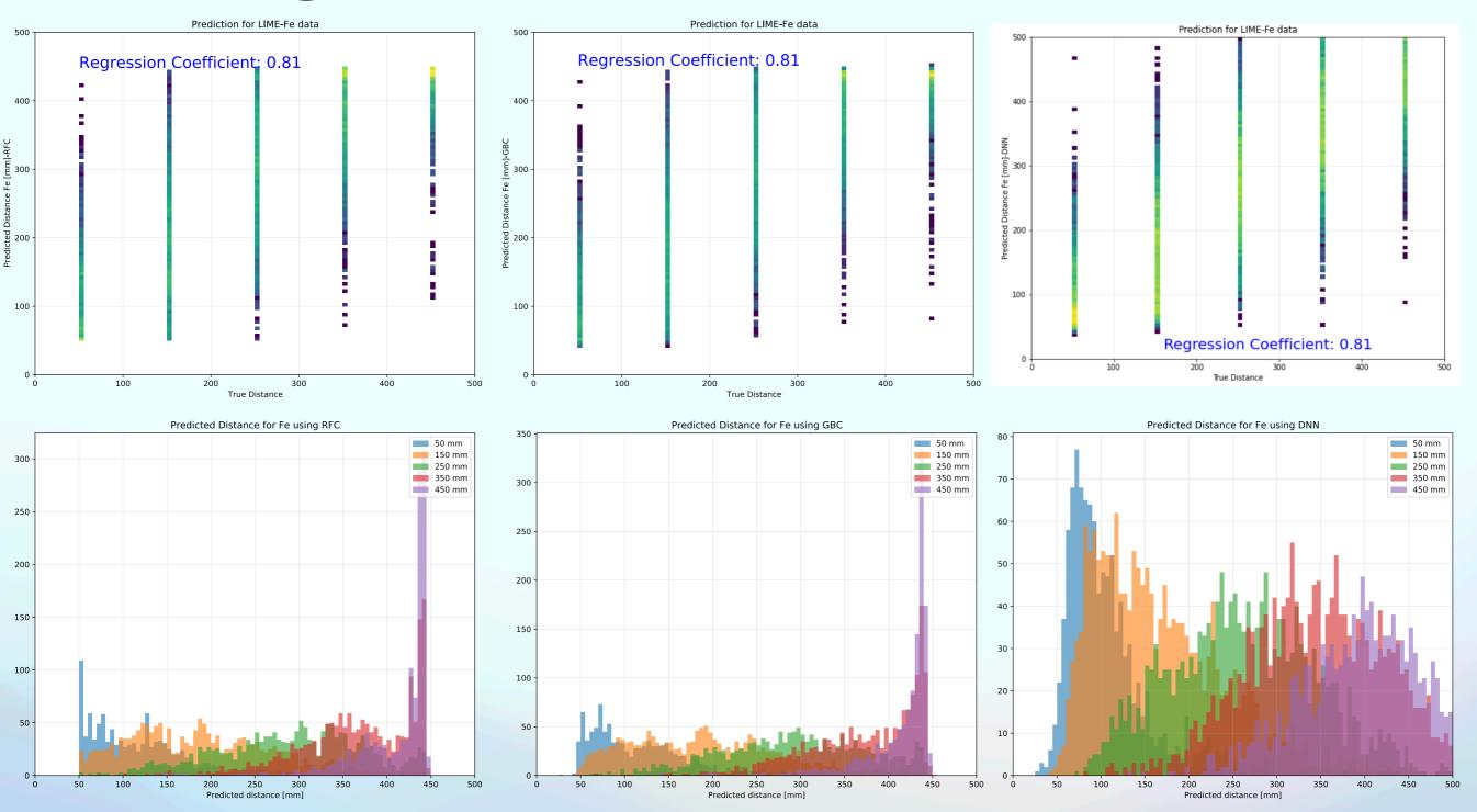
Prediction on MC is better because the z in MC does not have the spread like the Fe data.
