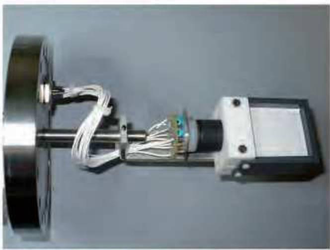
Fig. 2. Beam particle counter, based on a plastic scintillator coupled to a photomultiplier.
