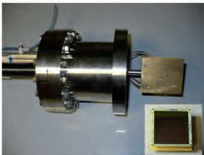
Fig. 3. PSSD mounted in a pneumatic actuator. The mask made by brass is 2mm thick.
