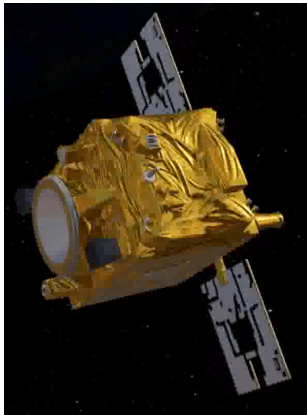
Microscope spacecraft wrapped with MLI
