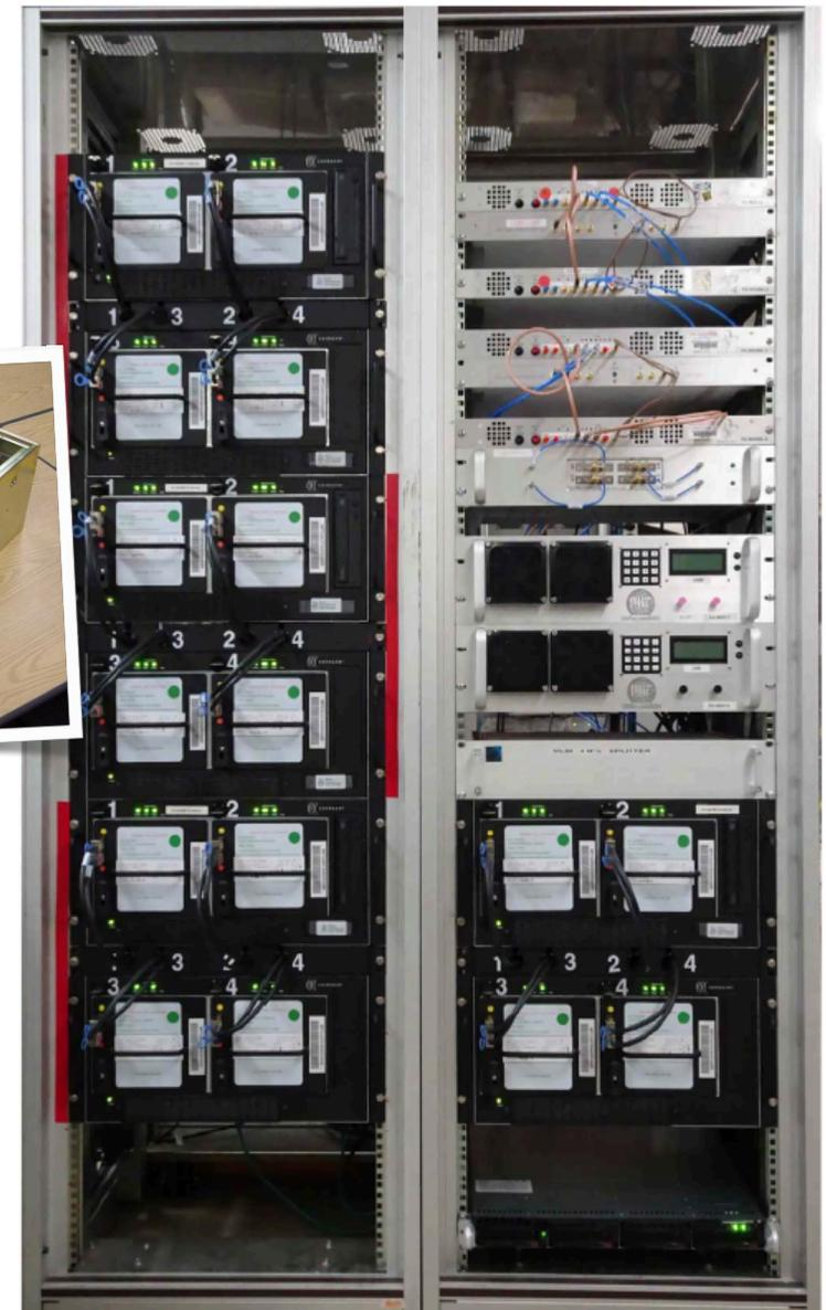
Figure 8. EHT digital VLBI backend as installed at the Institut de Radioastronomie Millimétrique (IRAM) PV 30 m telescope in Spain. The
