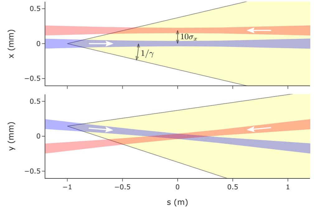
FIG. 27. The typical LHC interaction point (IP) configuration compared to a  $1/\gamma$  cone of gamma-radiation. The diameter of the beams in this picture is  $4\sigma_{x,y}$  (at the IP  $\sigma_{x,y} \approx 19 \mu\text{m}$ ). The beams are separated by  $10\sigma_x \approx 0.2 \text{ mm}$  horizontally in order to avoid stripping of the PSI due to collisions with counter-propagating ion or proton beam.
