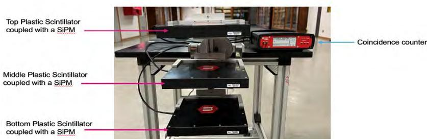
We have used three different layers so that we can get very precise data and understand if the signal is generated by a muon.
