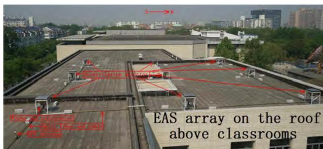
On the roof of Dongzhimen Middle School, a detector array is built to measure Extensive Air Shower (EAS), as shown in the above figure.
