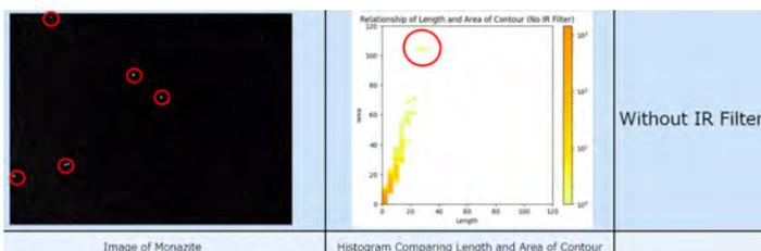
By removing a thin IR (Infra-red) filter that was on the sensor, we were also able to measure alpha radiation as can be seen in the image and graph.
