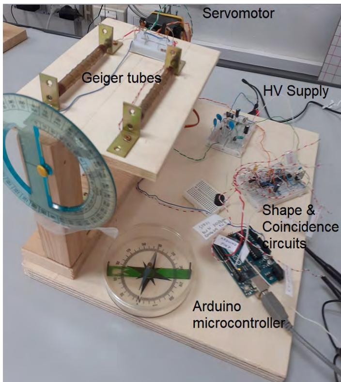
We used a home-built detector (muon telescope), already used last year, consisting of two SBM-20 Geiger tubes placed on a rotating tablet using a servomotor controlled by a PC via the Arduino microcontroller. The measurements can be carried out remotely by controlling the PC with the Teamviewer software.
