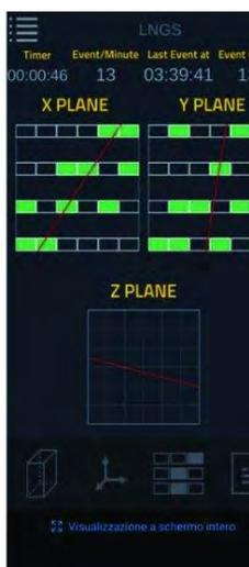
For each floor there are 6 rods aligned orthogonally to each other, to which your SiPM is associated.
