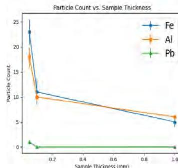
Fig.1 Diagram of our cloud chamber Fig.2 Photograph of cloud chamber Fig.3 An observed electron track Fig.4 Particle Counts vs. Sample Thickness
