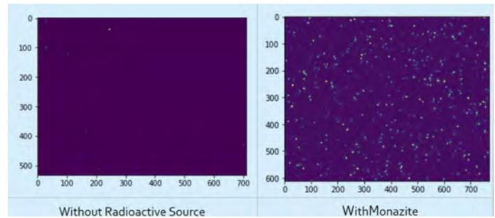
To measure radiation, we placed the radiation source in front of the sensor, then covered the camera with aluminum foil to block out visible light. You can see here some of the images we took with various radiation sources.
