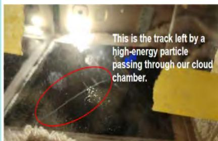
This portable hybrid cloud chamber can continuously observe cosmic rays in the air for a long period of time.
