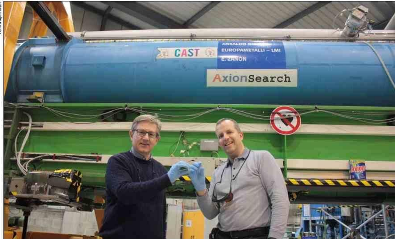
Giovanni Cantatore and Marin Karuza in front of the CAST magnet, holding the heart of the KWISP force sensor: nanomembranes to detect the direct coupling of exotic particles to matter.
