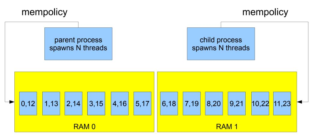
The host CPU scheduler understand the parent process has most of the RAM allocated in NODE 0 and the child in NODE 1 No scheduler hints from userland Mempolicy() doesn't have any scheduler effect
