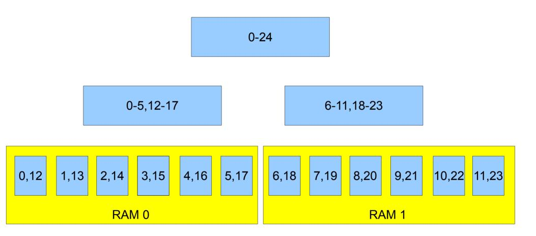
Example of a common 2 nodes, 2 sockets, 12 cores, 24 threads system
