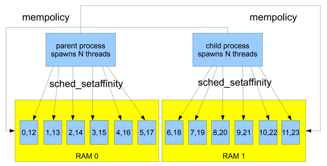
Worst possible CPU/RAM NUMA placement All CPUs only work on remote RAM
