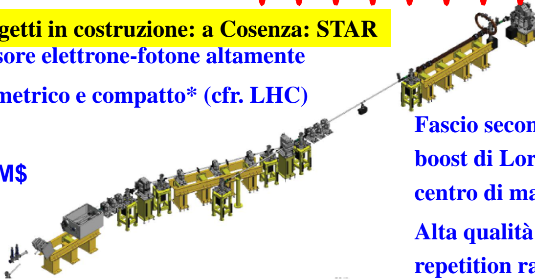
Fig.2 – STAR machine as an example of Paradigm A. Overall length about 12 m.
