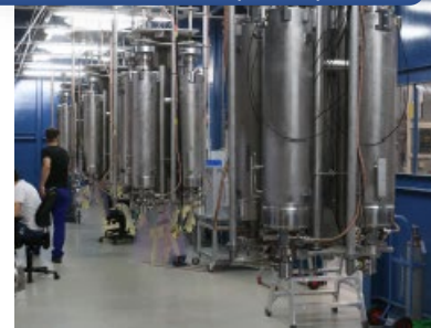
Cavities ready for the cold test at AMTF (DESY)
