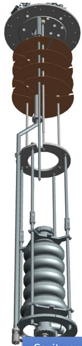
Cavity on insert with sensos and diagnostic installed
