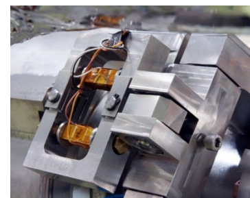
Piezoelectric actuators for fast tuning, E-XFEL, DESY
