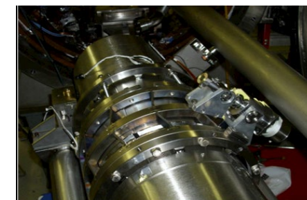
INFN Tuner for the ILC cryomodule at Fermilab, USA
