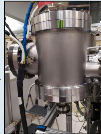
Vacuum chamber in stainless steel and has a cylindrical form with dimensions of 20 cm diameter and 30 cm of length. Magnetron source with 2-inch Ti target (99,99 %)
