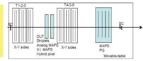
New flexibility implemented in DAQ system (Bologna) to test all the different DUT's
