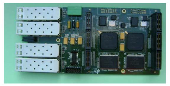
4 optical links at 1 Gbit/s; FPGA Xilinx, 40/100 MHz clk (programmable)
