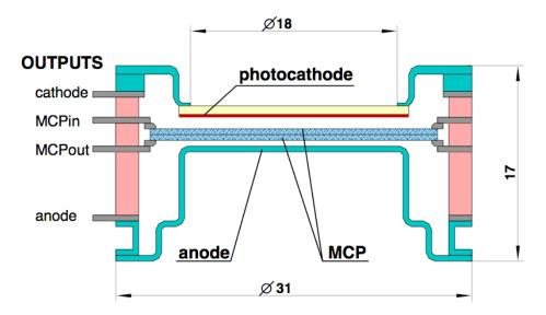
Manufacturer: "Ekran FEP" (Novosibirsk) Borosilicate glass window Multialkali (Sb-Na-K-Cs) photocathode Maximum QE at  $\lambda$ =500nm Two MCPs with channel diameter of 7 µm Channel bias angle 13° Single anode
