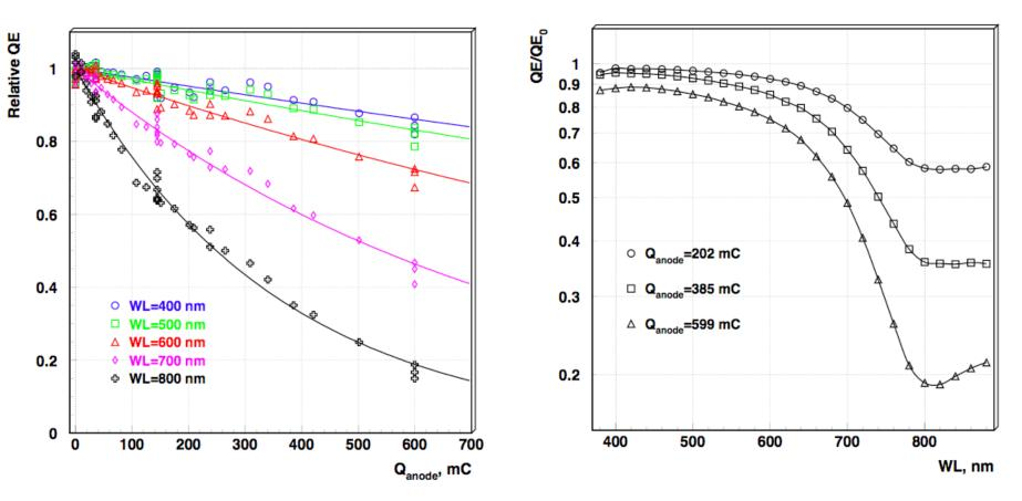
Possibility to control photocathode aging after short exposure not damaging QE in the 'working' region
