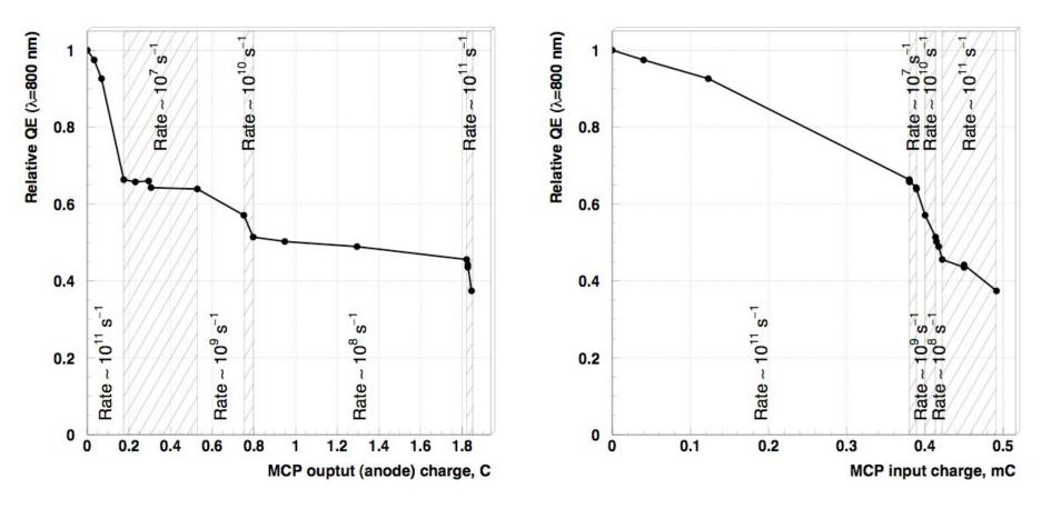
The higher counting rate the faster QE degradation per unit of anode charge The higher counting rate the slower QE degradation per unit of cathode charge
