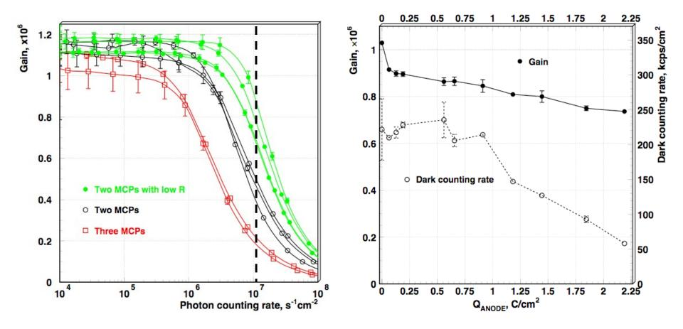
Lifetime measurements at counting rate of 10<sup>7</sup> s<sup>-1</sup>cm<sup>-2</sup> where gain decreases by 20-30%
