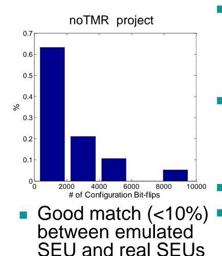
Total of 19 runs 18 runs @ 6 Gy/min (Si) 1 @ 23 Gy/min (Si) Avg. duration 146 s => total dose per run 14 Gy (Si) We measured # of configuration bit-flips accumulated before link failure (error burst) (N<sub>flips</sub>) On average N<sub>flips</sub> =2070 During the SEU emulation tests performed in lab. in May, N<sub>flips</sub>=2250
