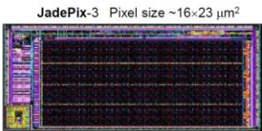
Tower-Jazz 180nm CIS process Resolution 5 microns, 53mW/cm²
