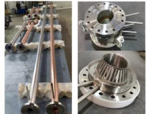
Vacuum pipes and RF shielding bellows
