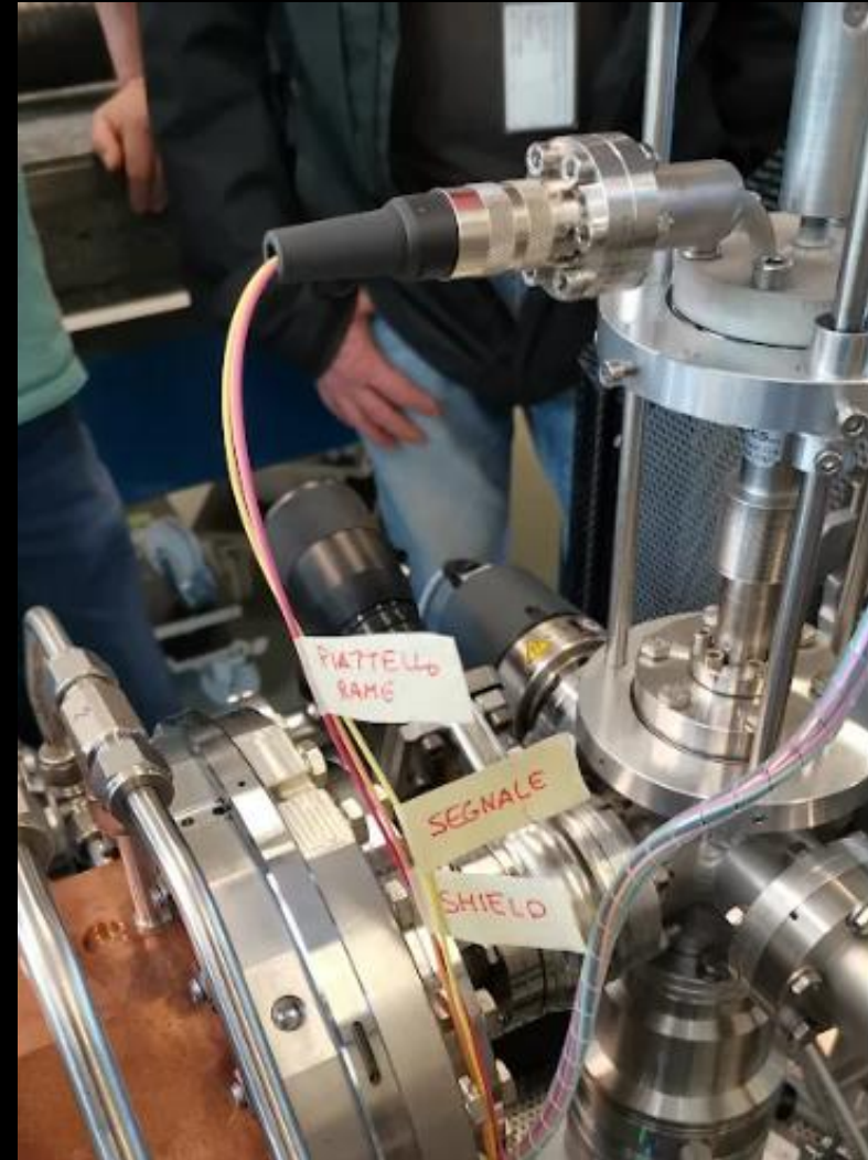
Connector and cable for screen, guard ring and Faraday cup Middle: 50 mm long bellow for axial movement
