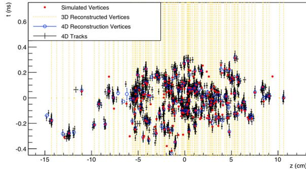
Fig. 1.: Simulated and reconstructed vertices in a bunch crossing with 200 pileup interactions assuming an MTD resolution of  $\sim 30$  ps. Simulated vertices are reported as red dots; 3D-reconstructed vertices are drawn as vertical yellow lines, while 4D-reconstructed tracks and vertices are drawn as black crosses and blue open circles.
