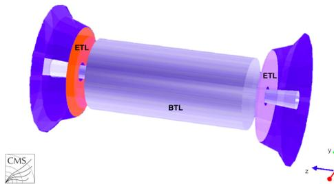
Fig. 3.: Schematic view of the GEANT geometry of the timing layers, including a barrel layer (grey cylinder), at the interface between the tracker and the ECAL, and two silicon endcap (orange and light violet discs) timing layers in front of the endcap calorimeter.
