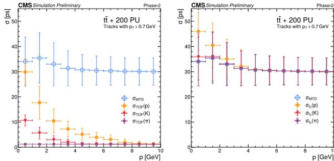
Fig. 4.: On the left, estimated MTD hit uncertainty  $\sigma_{\text{MTD}}$  (blue) compared to  $\sigma_{\text{TOF}}$  under the pion (purple), kaon (red) and proton (orange) hypotheses. On the right,  $\sigma_{\text{MTD}}$  is compared to the total track time uncertainty  $\sigma_{t_0}$  as obtained from Equation 4. For each momentum bin, the mean value and standard deviation of the distribution is shown.
