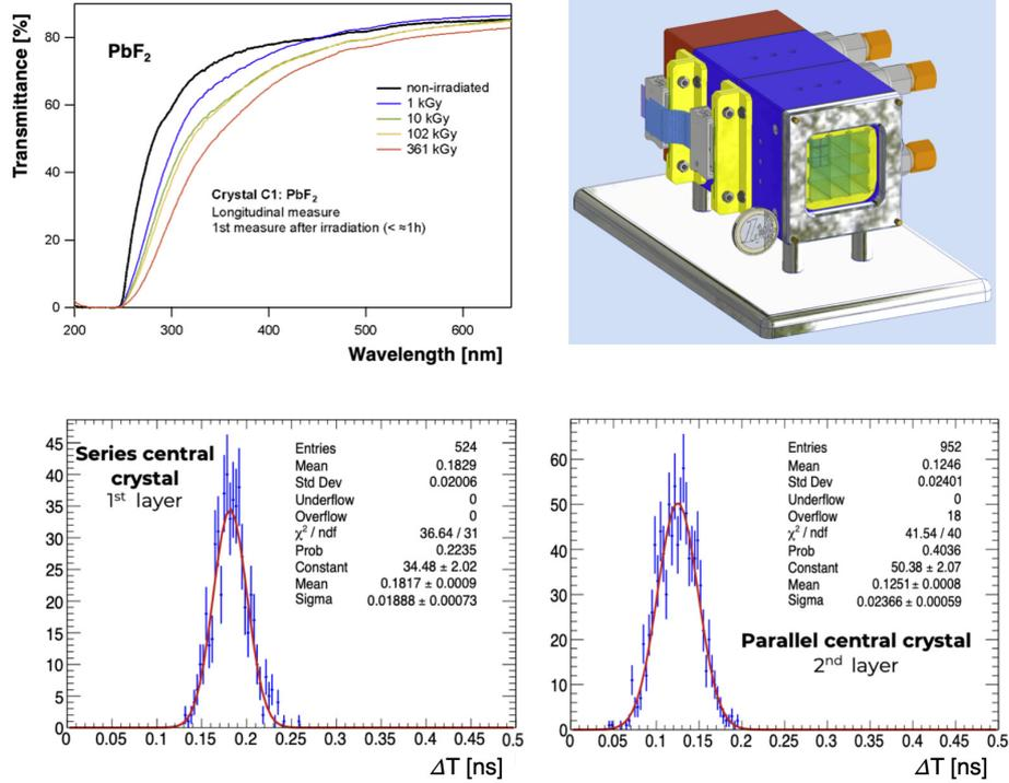
Fig. 3.: Top left: Transmission spectra obtained at various irradiation stages. Top right: 3D proto-1 overview. Bottom: Gaussian fit of  $\Delta T$  distributions for the central crystal of first layer (left) and second layer (right).
