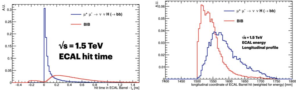
Fig. 1.: Left: Timing of ECAL barrel hits relative to the bunch crossing time for BIB (Red) and  $H \rightarrow b\bar{b}$  signal (Blue). Right: Distribution of the energy of the ECAL barrel hits respect the distance from the beam axis, for BIB (Red) and  $H \rightarrow b\bar{b}$  (Blue).
