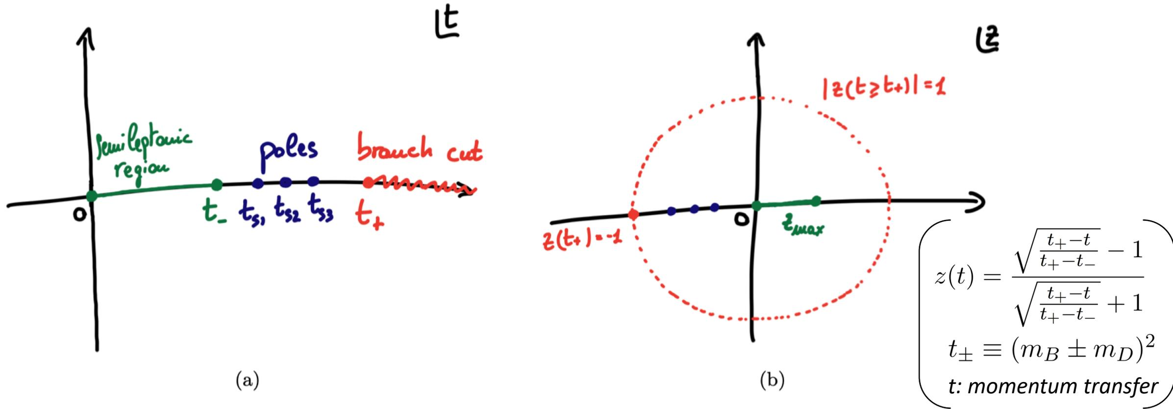
Figure 3.3: Sketch of the analytic structure of the hadronic form factors as function of  $t$  (left panel) or as function of  $z$  (right panel). The green line represents the region relevant for semileptonic decays. The blue points are the isolated poles coming from one-particle states. In conclusion, the red branch cut in the left panel is caused by multi-particle states, *i.e.* states of two or more particles. This branch cut translates in the unit circle  $|z| = 1$  in the right panel.
