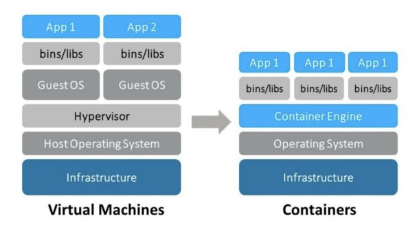
The Containers work on the concept of **OS-level virtualization**, i.e. the kernel's ability to make multiple isolated environments on a single host.
