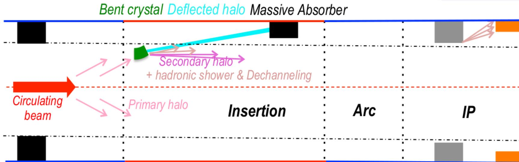
Working principle of a crystal collimation system [33]
