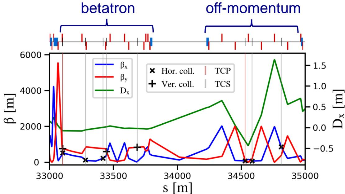
FCC-ee beam halo collimator parameters and settings
