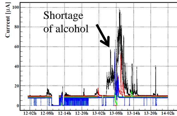
Current spikes solved by **addition of oxygen and isopropyl alcohol**
