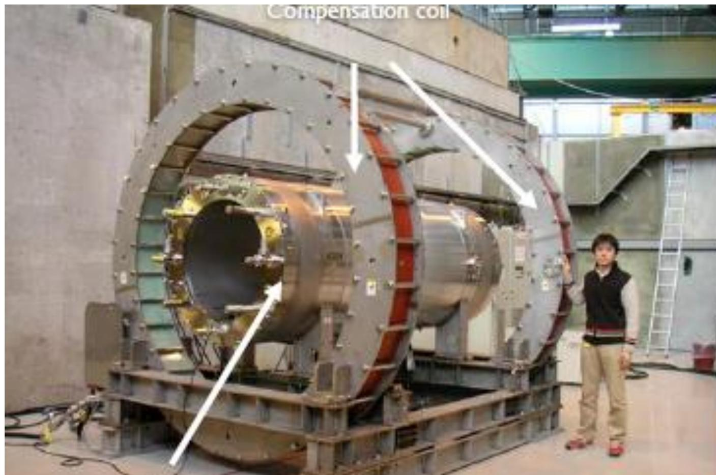
Superconducting solenoid with gradient field (**COBRA**).
