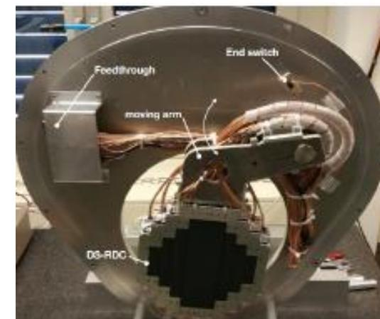
Lyso plastic scintillator array read by SiPM.
