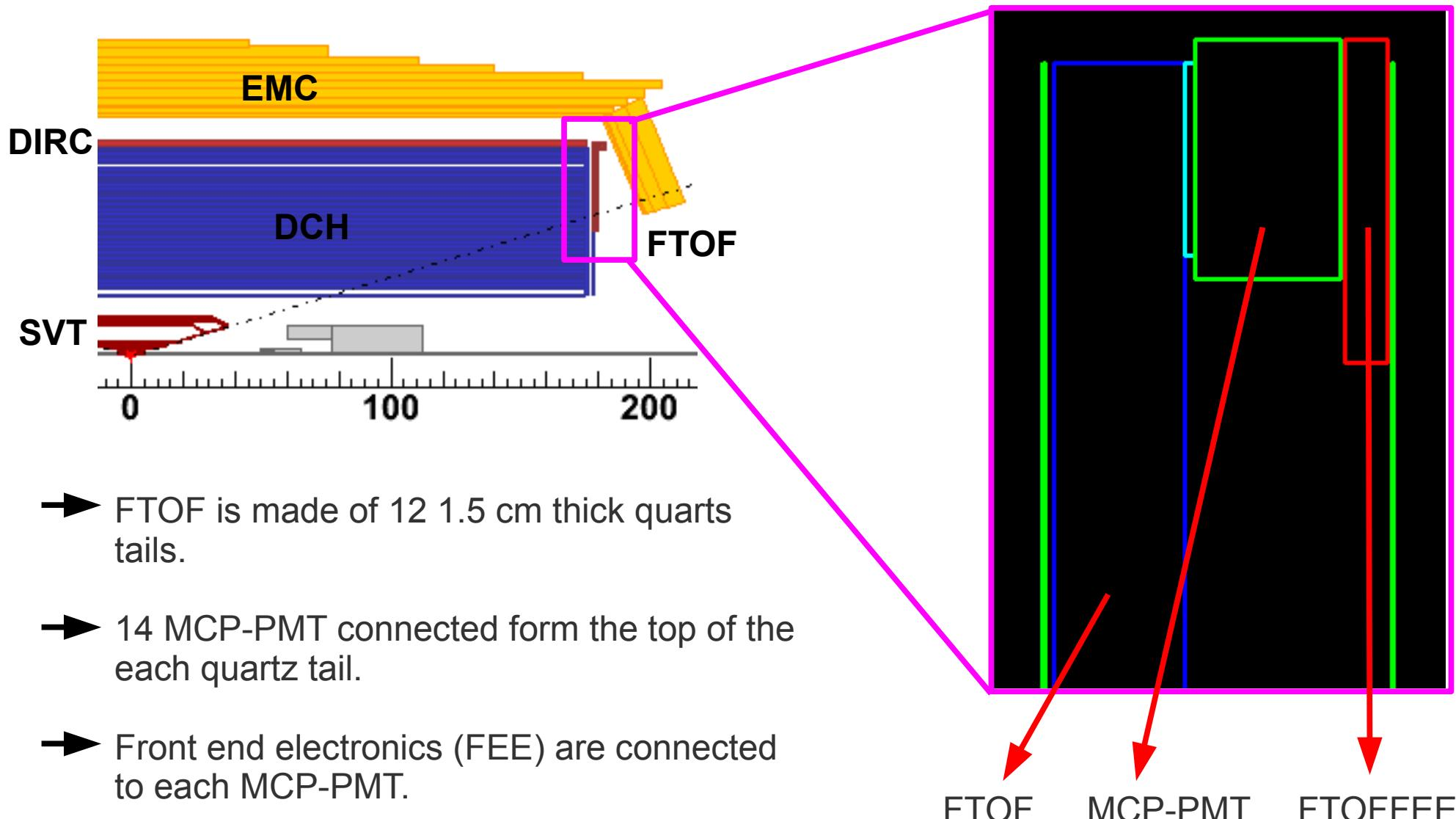
FTOF      surface  $\sim 1.87 \times 10^4 \text{ cm}^2$ , mass = 61.7 kg ( $\rho=2.2 \text{ g/cm}^3$ )
