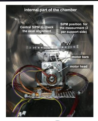
Internal view of the chamber with the motor installed, moving support with 5 SiPMs and 3 Pt100 to monitor temperature and liquid level.
