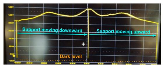
SiPM integrated signal (luminosity) during support movement (40 cm): signal is constant within ~30% and reproducible in the two directions.
