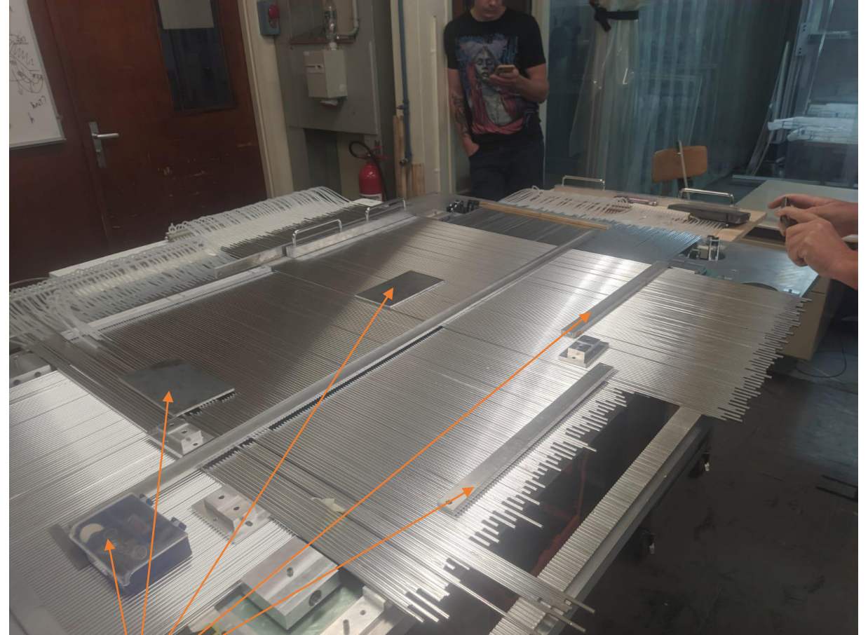
Weight keep in position straw tubes during assembly
