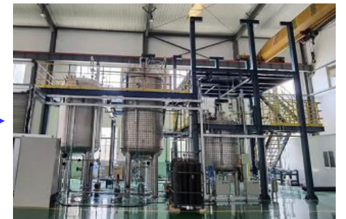
Mixing LAB with PPO and bis-MSB
