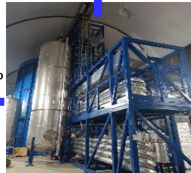
4) Gas stripping to remove Rn and O 2
