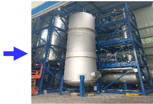
2) Distillation for radiopurity
