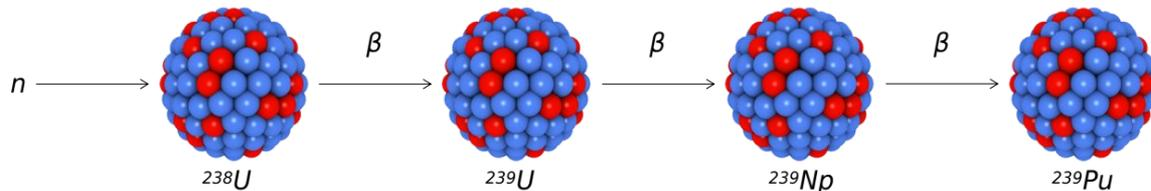
Most of the enriched  $^{235}\text{U}$  fuel in a reactor core is in fact  $^{238}\text{U}$ , which can be converted  $^{239}\text{Pu}$ .
