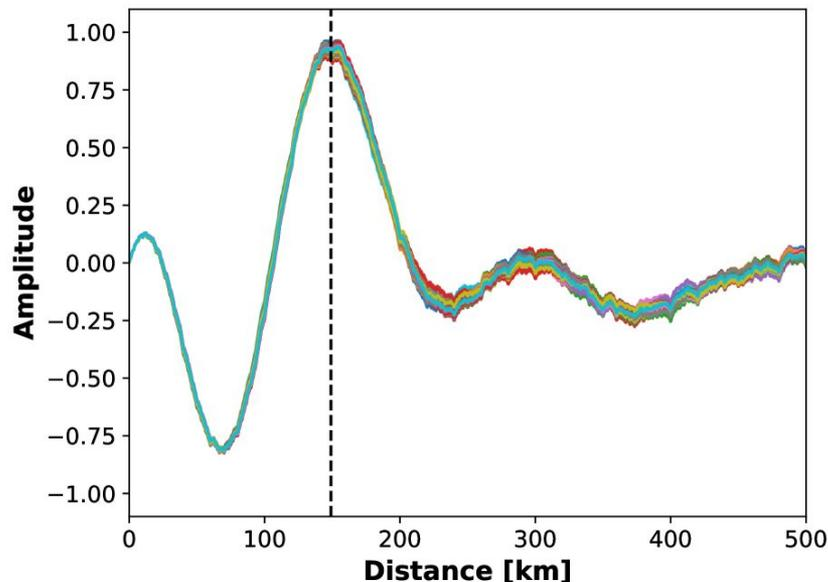
Fourier transform converts energy spectrum to distance to reactor.
