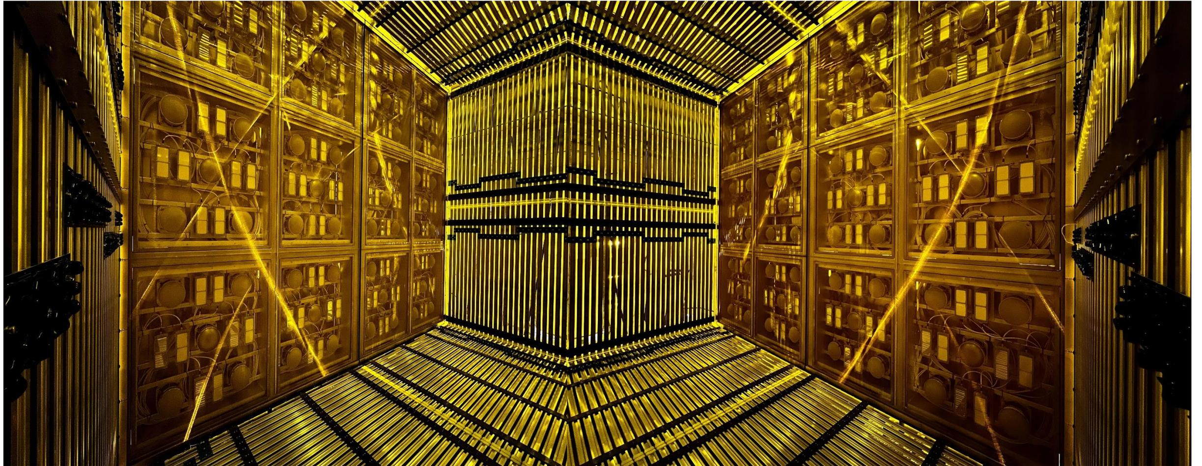
**196 small X-ARAPUCAs installed in the SBND detector at Fermilab**
