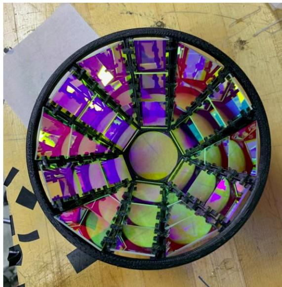
Winston cone made of flat dichroic filters => concentrate long wavelenrgths and pass short wavelength
