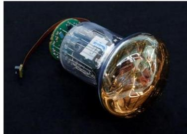
**Glass sphere containing 31 3" PMTs, onboard calibration and readout electronics**
