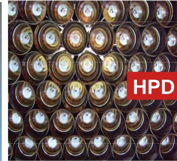
*Large area Photocathode coupled to an APD in vacuum*
